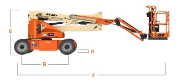
A. Platform Width 30-in / 76-cm B. Platform Length 60-in / 1.52-m C. Machine Width 5-ft 9-in / 1.75-m Tailswing 0-in / 0-cm E. Machine Height 6-ft 7-in / 2.01-m F. Machine Length 21-ft 2-in / 6.45-m G. Wheelbase 6-ft 7-in / 2.01-m H. Ground Clearance 8-in / 20-cm
